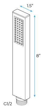
Flow Rate: 2.0 GPM / 7.6 LPM
